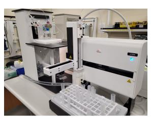
Figure 6. AccuSizer APS system (left) and autosampler (right).
