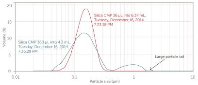
Figure 6b. Laser diffraction spiked CMP result.
