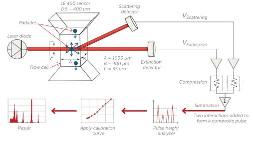
Figure 2. LE400 sensor/counter diagram.
