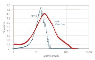
*Figure 4. The AccuSizer system builds the distribution one particle at a time, providing accurate results.*
