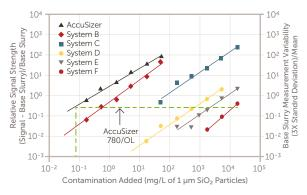
Figure 5. SiO<sub>2</sub> particle detection study.
