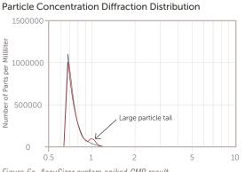
Figure 6a. AccuSizer system spiked CMP result.
