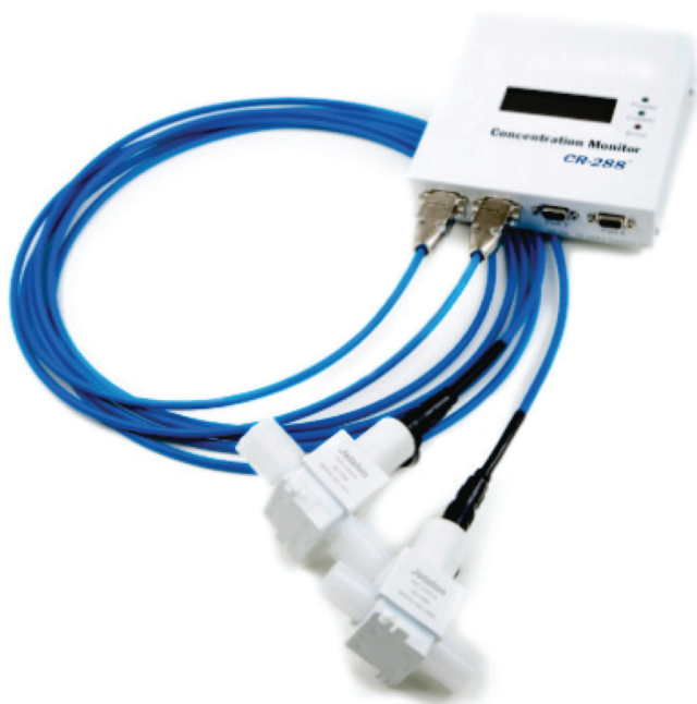
Figure 1. Index of refraction analysis system. The analyzer sensor head contains a miniaturized optical sensor that is in contact with the liquid chemicals under analysis.
